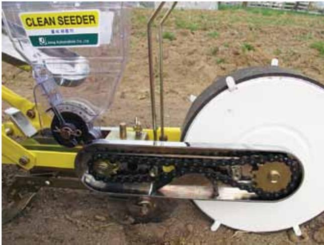
The Jang seeder has interchangeable rollers with holes drilled to singulate seed. It is shown here with the cover removed to show the gears that can be changed to adjust seed spacing.
