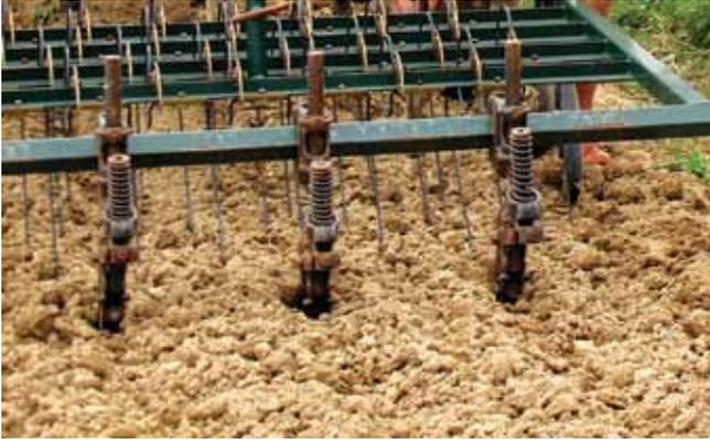
Row-marking knives mounted on a tool bar mark straight rows that can be used to guide seeding with a push seeder or hand transplanting. This allows for straight enough rows for mechanical cultivation. Marking knives are shown mounted on Williams Tools System tool bar at Quiet Creek CSA, Kutztown, Pa.
