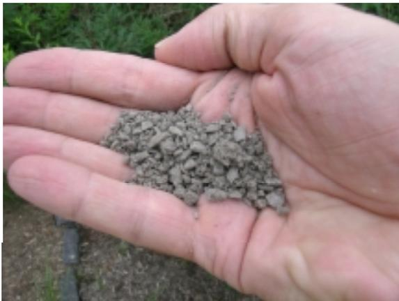
**Figure 1. Typical calcitic limestone sand used for direct application to streams.**
